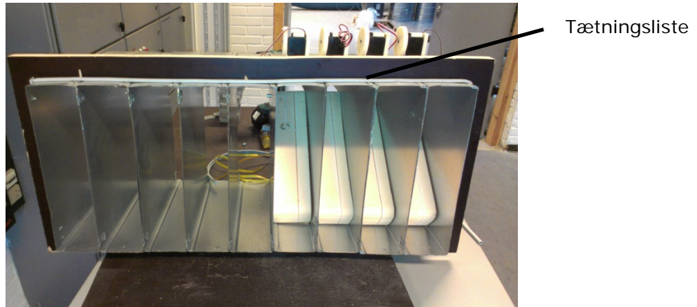
Figur 4-22: Prototype manifold set fra ventilatorsiden.
