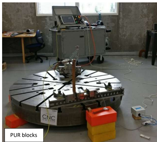
Figure 1 Set-up used for VSR treatment of medium and small parts which require a fixture on a plane supported by 3 polyurethane (PUR) blocks.
