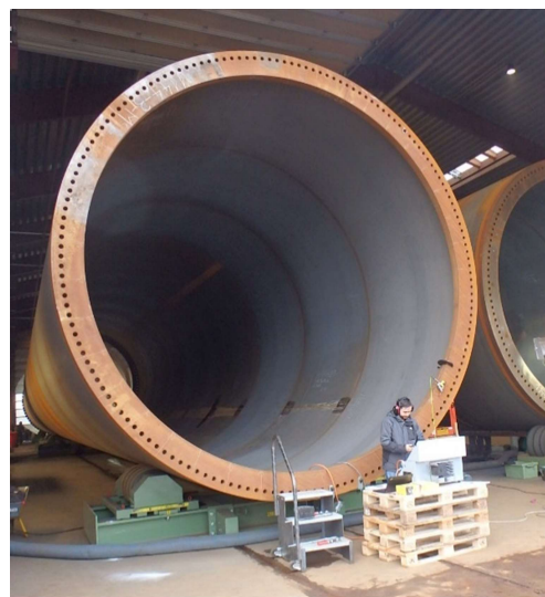
Figure 3 Test of vibrations on part 2, a 126 ton tower section for a wind turbine.
