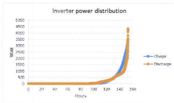
Figure 5: Measured distribution curve of the battery inverter power in May. It appears that there are very few operating hours above 3 kW which is only half of the maximum output power of the battery inverter.
