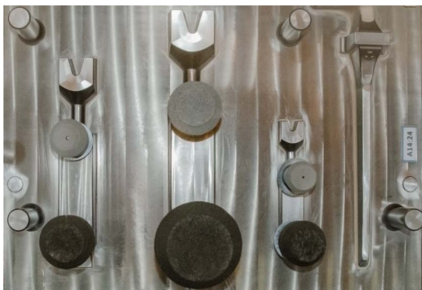
Fig.4: Spot feeders from group 6 mounted on the pattern, ready for moulding. Insulating spot feeders on the top. Exothermic spot feeders at the bottom.
