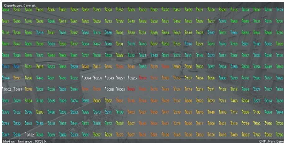
Figure 3 Rendering output of outdoor environment with a CIE overcast sky
