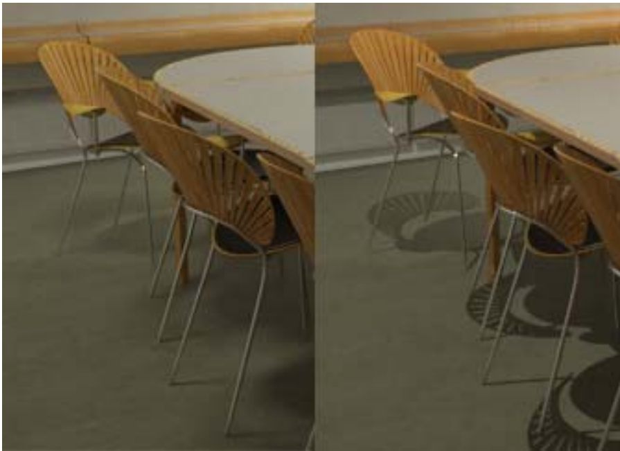
Figure 6 Comparison of the far field photometry problem in a standard IES file (right) and the approximate grid divided area light shape used to counter this (left).
