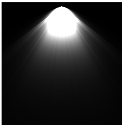
Figure 5 A sample IES file from a luminaire
