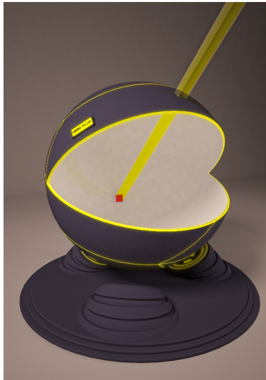
Figure 1 3D simulation of the integrated sphere used in the validation experiment (diffuse reflectance characterization). The light is being directed "through" the outer shell of the sphere
