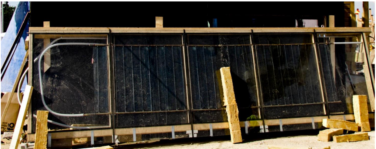
Figure 20 – Photograph of the solar thermal collector module before its mounting on the Weather Shield
