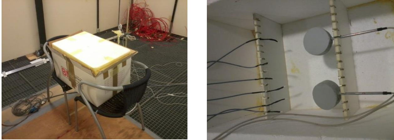
Figure 101 – Sensors calibration : outside and inside the insulated box used for the calibration
