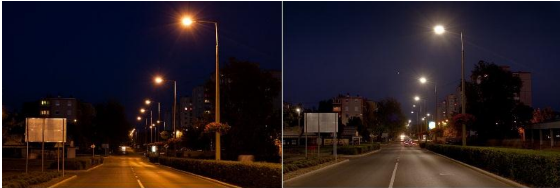
Figure 3: Kaszap Road, replacement of HPS by LED (© City of Hódmezővásárhely, Tungram-Schröder)
