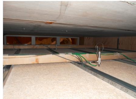
Fig. 5. Temperature and velocity sensors in the moveable columns. (a) Without diffuse ceiling. (b) With diffuse ceiling.
