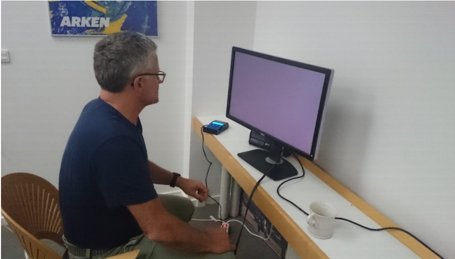
Figure 5-4 Test setup using a monitor as glare source, with target in the centre
