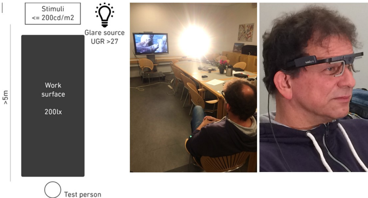
Figure 5-13 Configuration used in pilot study 4, with observers looking at a fixed image or a movie on a screen located 5 meters in front of her/him. The study was conducted for a horizontal illuminance of 200 lux and with or without glare source (UGR around 27)
