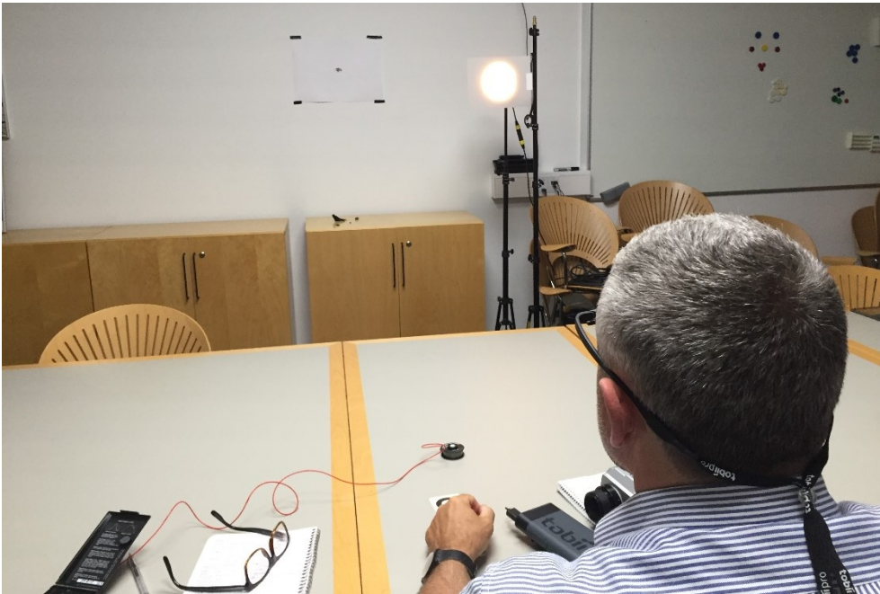
Figure 5-8 Test setup with glare source close to gaze point
