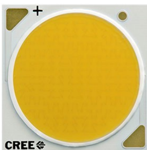
Figure 1-2 Cree XLamp CXB3590, 4,000 K, CRI 70, Light emitting area \varnothing 28.5 mm. This component provides approximately 13,000 lumen @85°C – or more than 16 traditional incandescent 60W lamps (Photo: Cree)
