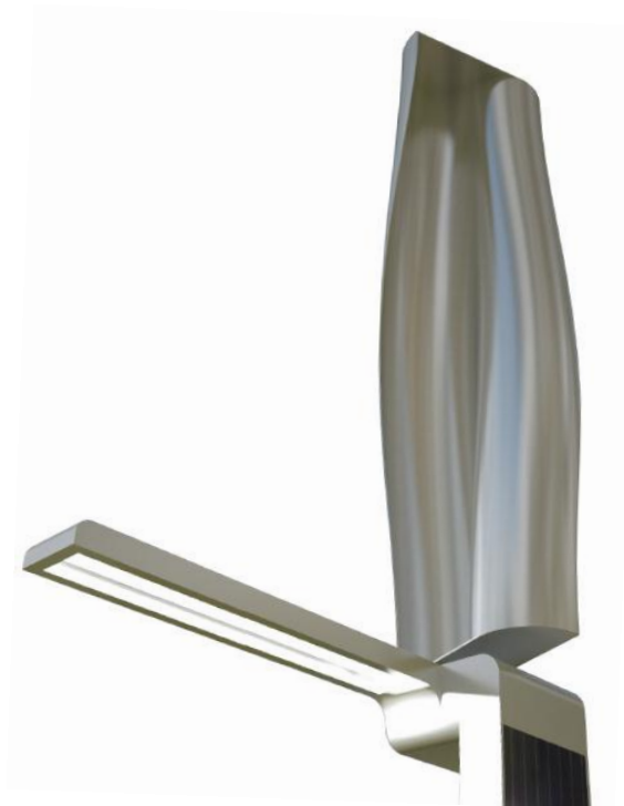
Figure 55: Present design 90-degree twist Savonius turbine with small end plates at the top and bottom of the turbine, visualized with the LED luminary underneath the turbine
