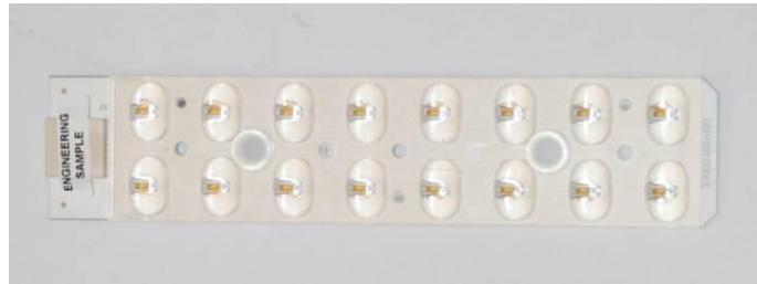
Figure 49 – LEDgine module from Philips
