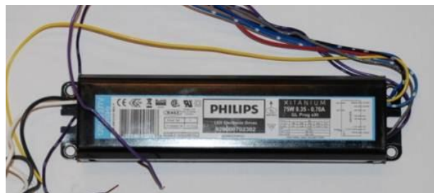
Figure 50 – Programmable LED driver from Philips Lighting
