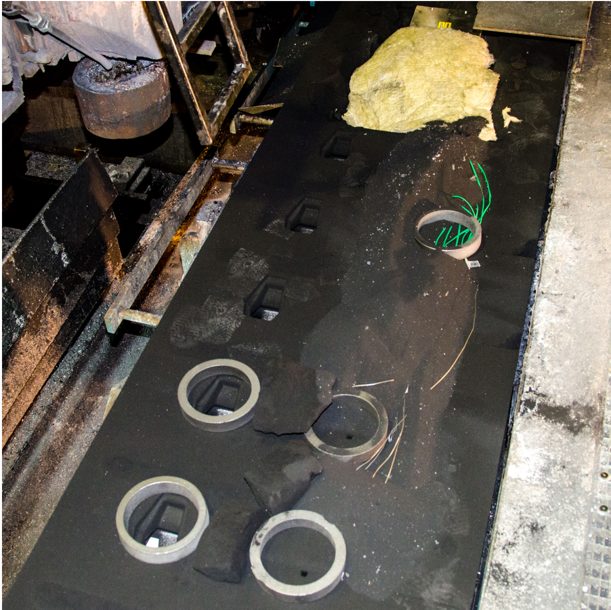
Figure 12.8: Overview of the TC setup and mould placement of castings 10A, 10B, 10C, and 17A.
