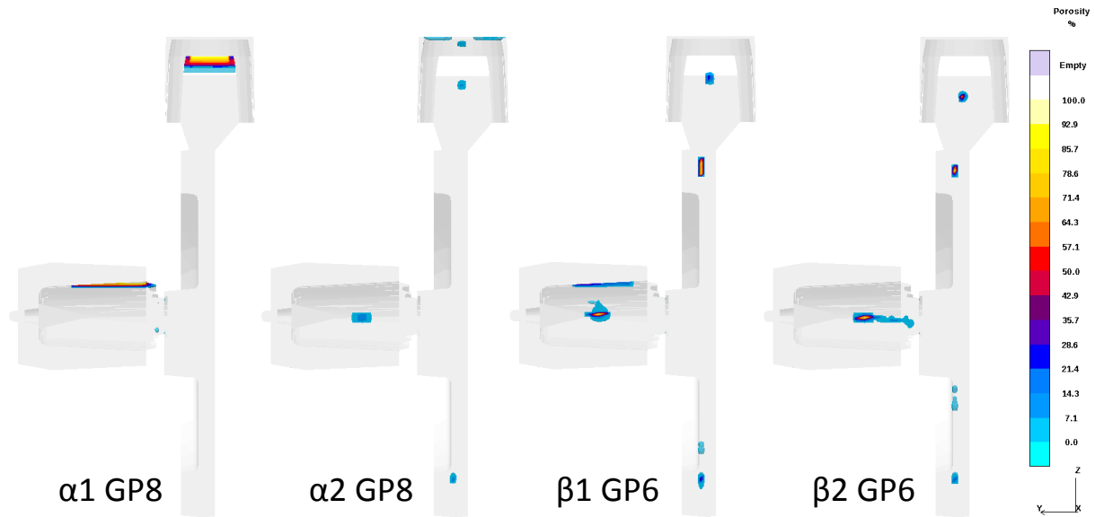
Fig. 6. These are porosity simulations for casting groups \alpha 1 , \alpha 2 , \beta 1 and \beta 2 . The 3D model is sectioned through the vertical centerline, exactly as the real castings were. The simulations of \alpha 1 and \alpha 2 apply a graphite precipitation factor of 8, and the simulations of \beta 1 and \beta 2 apply a factor of 6.
