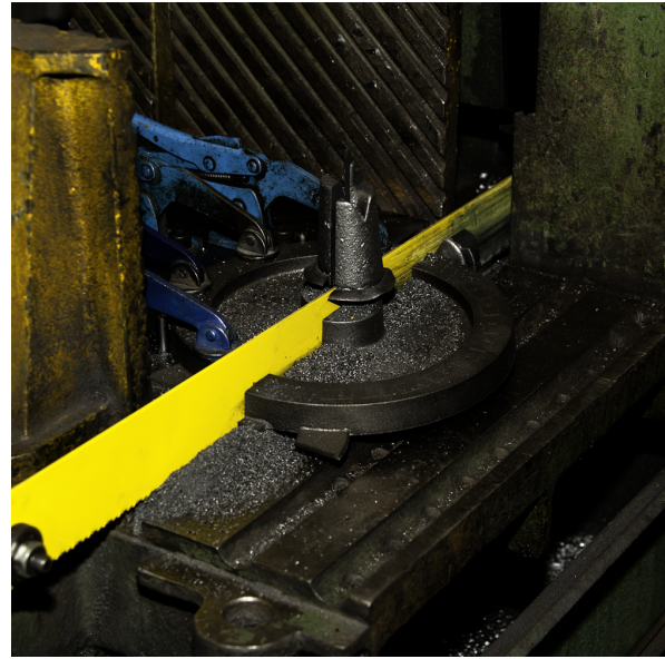
(b) All castings were first sectioned through the vertical centreline.
