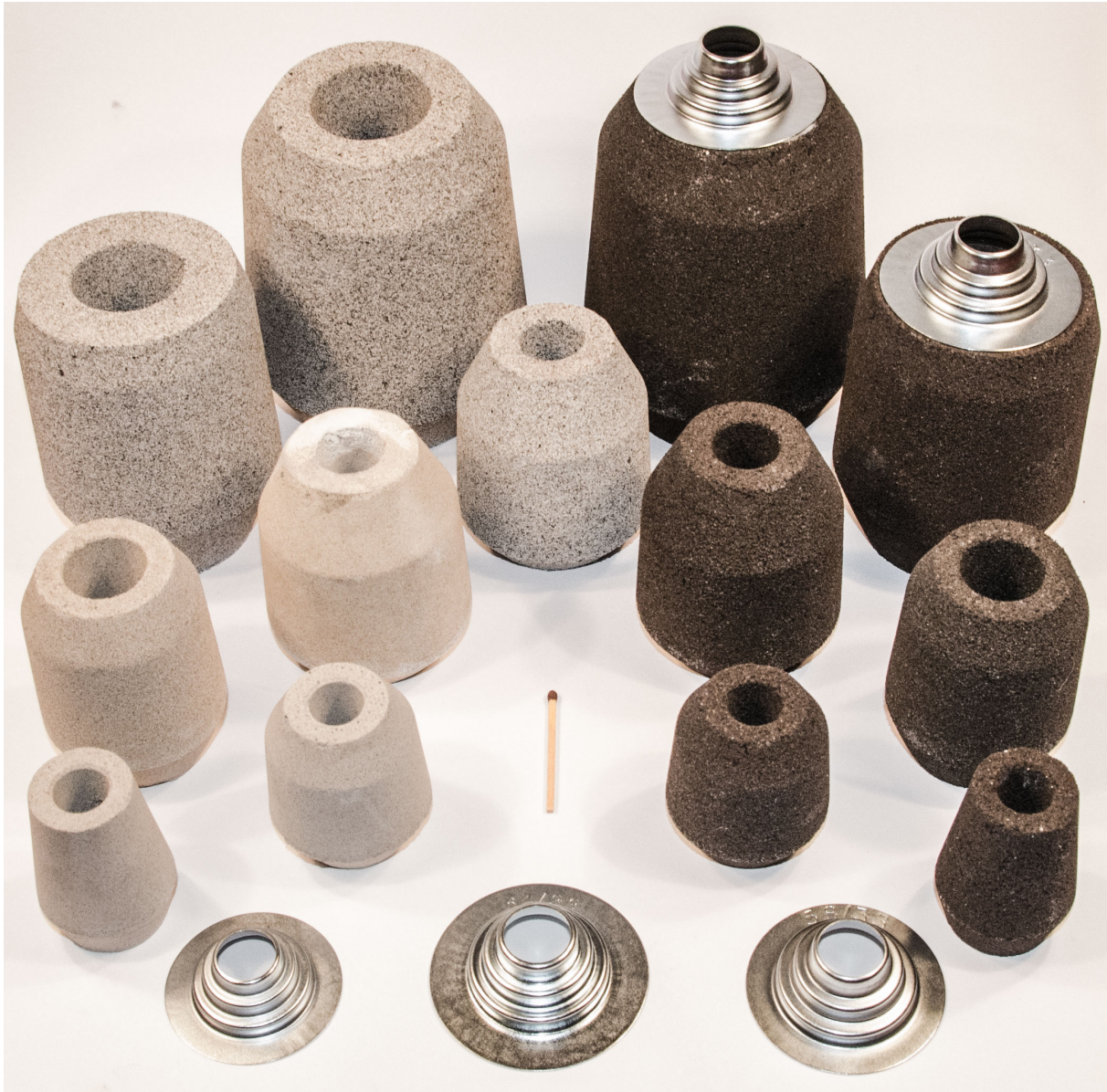
Figure 11.11: Insulating and exothermic versions of the selected Feedex HD V feeders, with the three sizes of metal breaker cores used for the trial.
