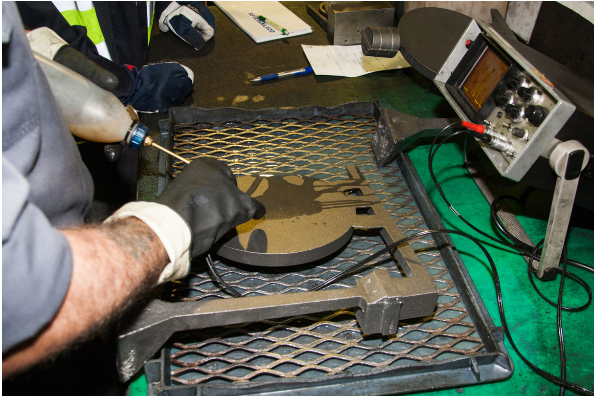
Figure 5.4: Ultrasound analysis of casting without centre feeder, before the sectioning.
