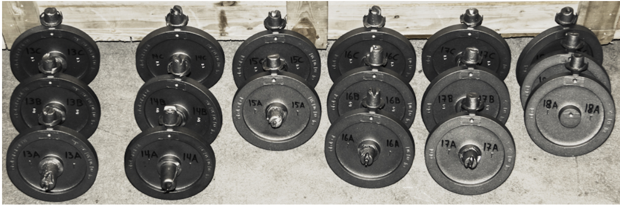
Figure 4.4: Overview of castings from session three. The missing casting, 15B, was incompletely filled during casting and was thus discarded.
