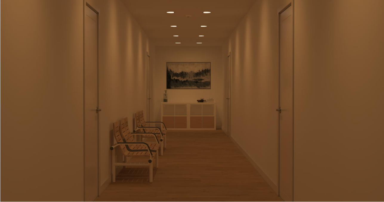
FIGURE 57. Hallway, Wallwasher 60 lux, FSL
