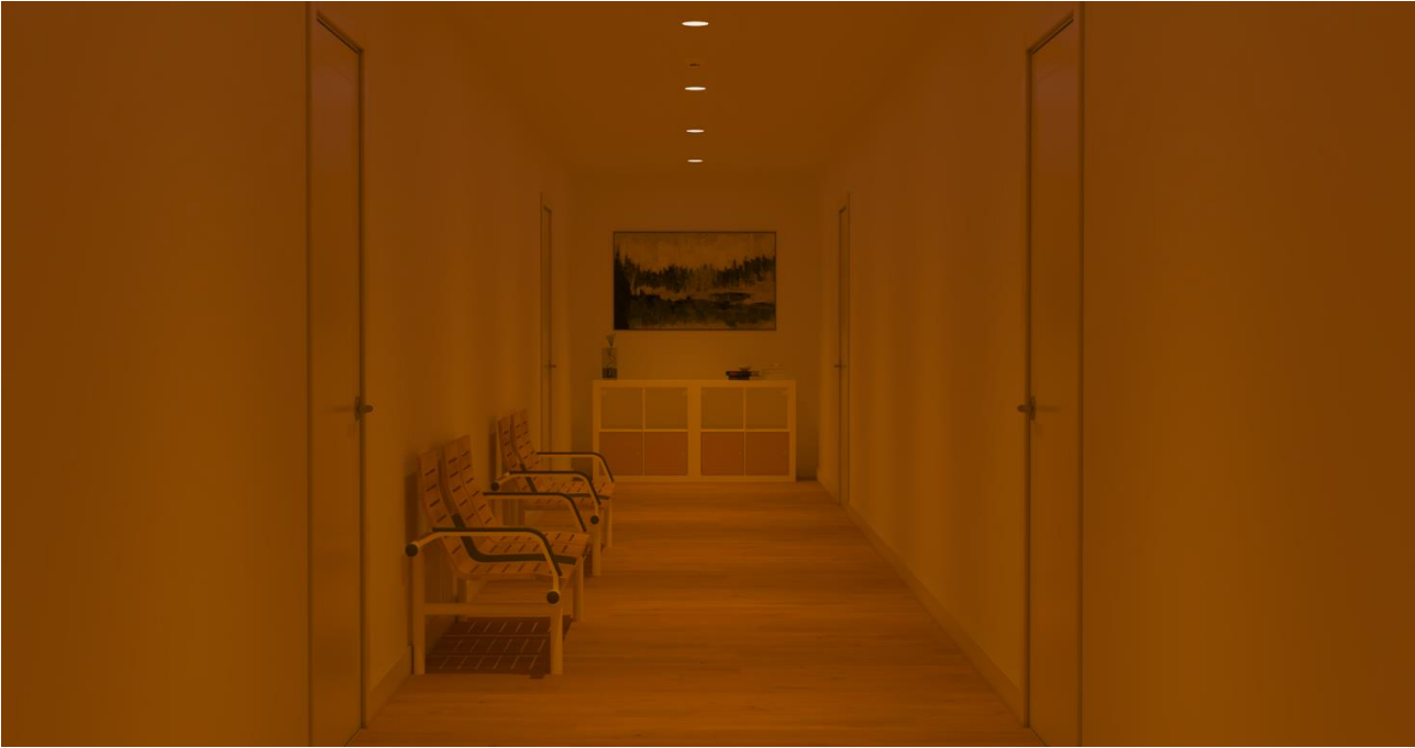
FIGURE 59. Hallway, Downlight (reference) 50 lux, RSL
