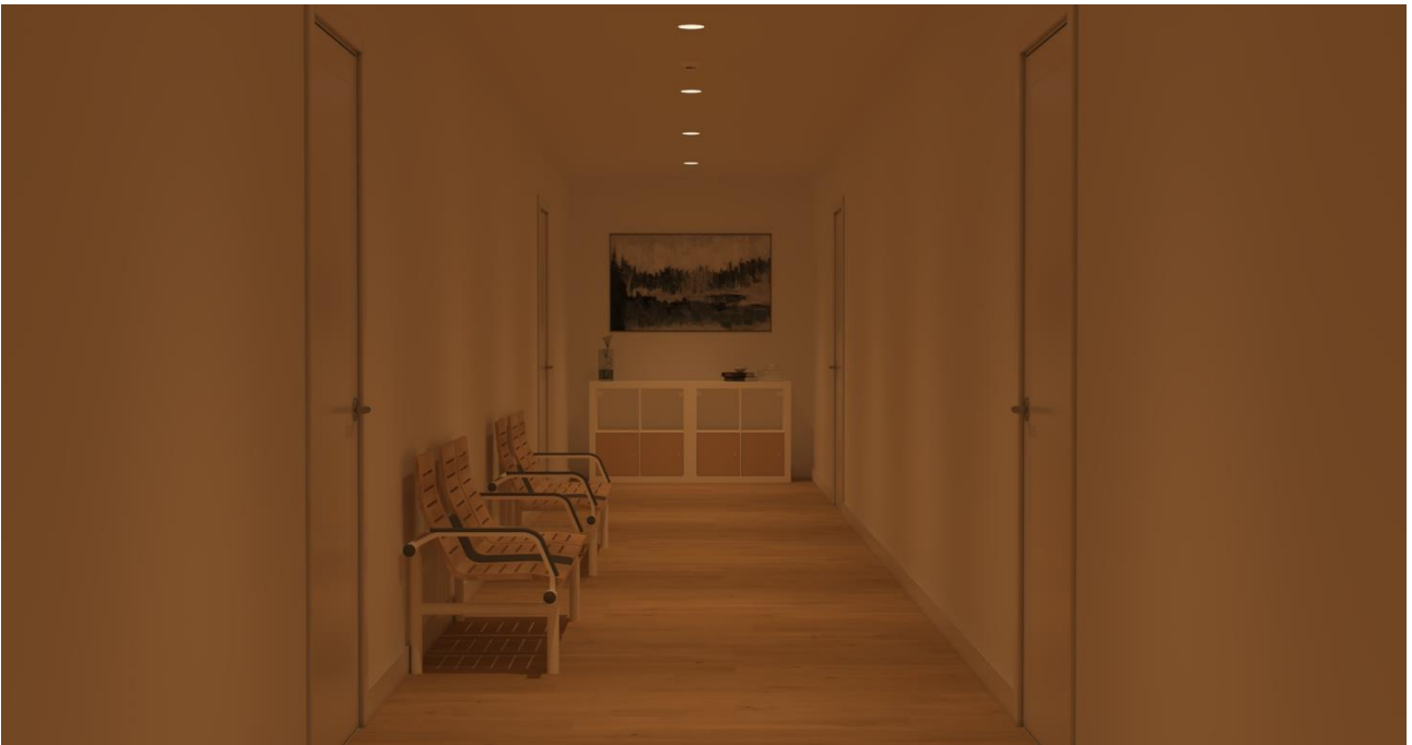
FIGURE 52. Hallway, Downlight (reference) 50 lux, FSL
