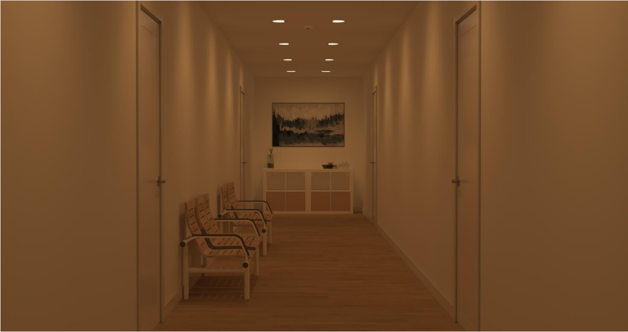
FIGURE 56. Hallway, Wallwasher 50 lux, FSL
