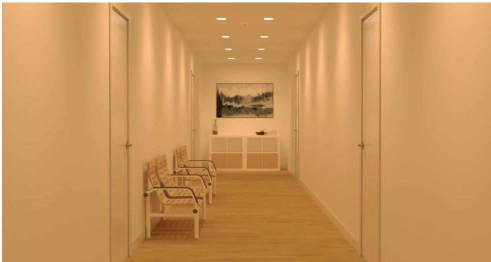
FIGURE 12. One of the visualizations of the hallway – Scene with wallwashers in FSL 3000K providing 50lx average horizontal illuminance on the floor.
