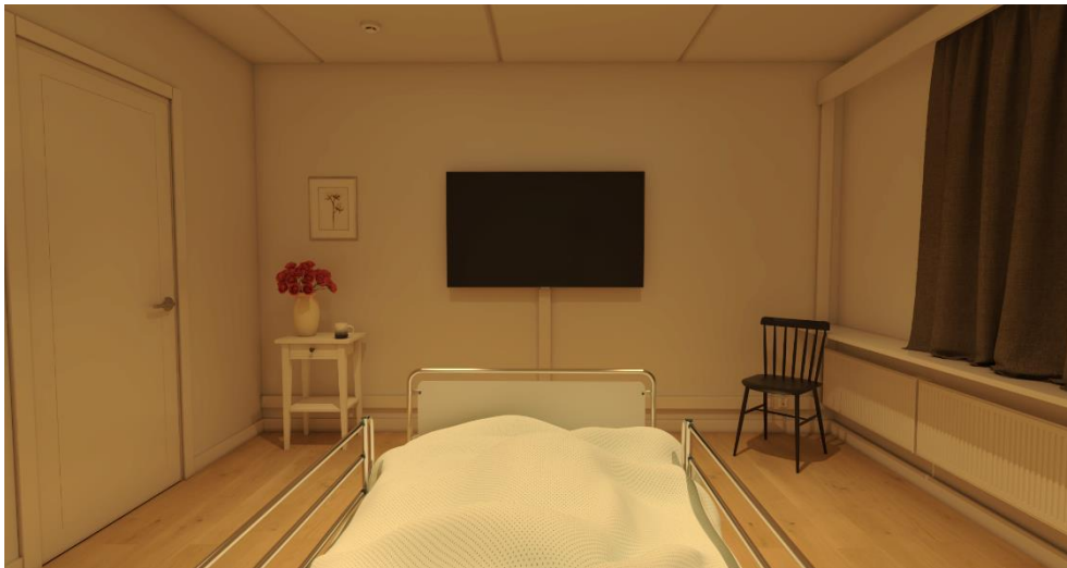
FIGURE 8. One of the visualizations of the patient room – reference scene with downlights in FSL 3000K providing 50lx average horizontal illuminance on the floor level.
