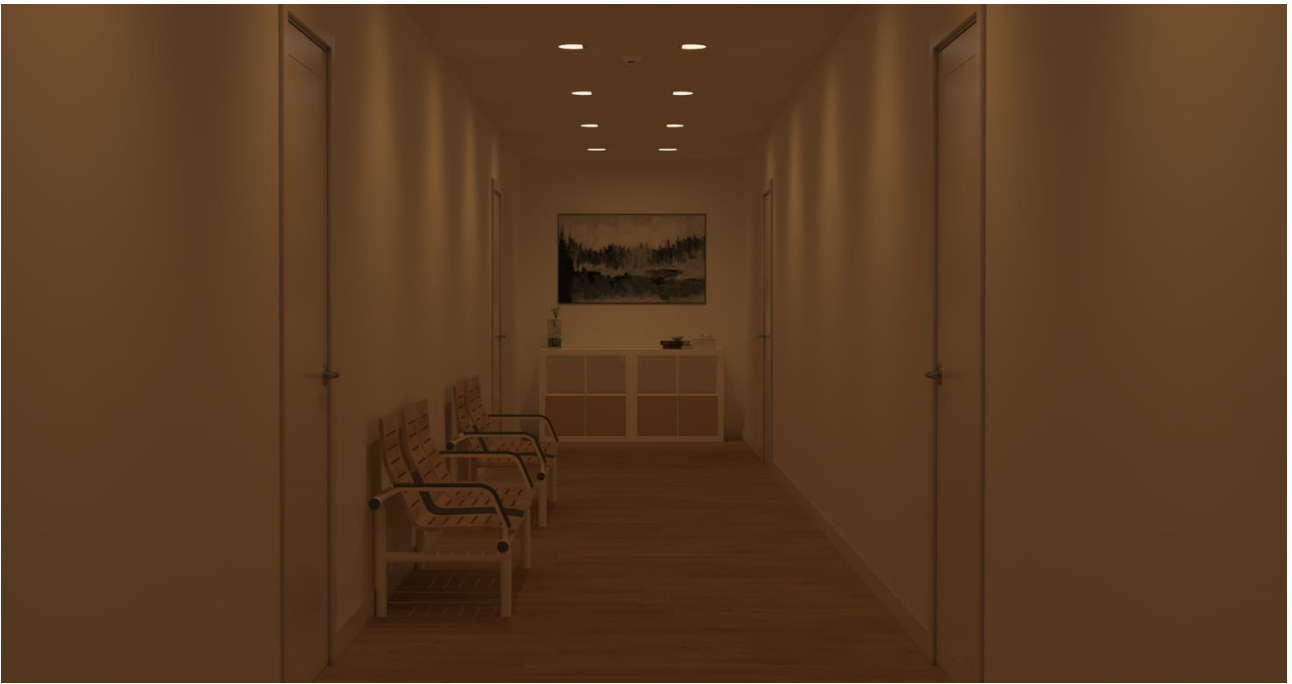
FIGURE 54. Hallway, Wallwasher 30 lux, FSL
