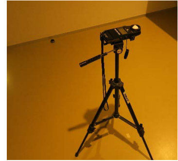
Figure 1-9 - Konica Minolta CL-200 illuminance and chroma meter
