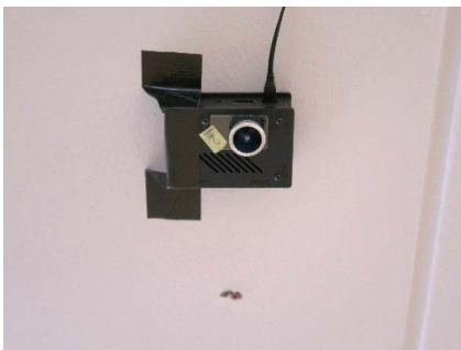
Figure 1-4. The sensor, Raspberry Pi computer with camera and fisheye lens
