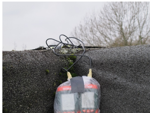
Figure 2-11 – Placement of the exterior illuminance data loggers on the roof
