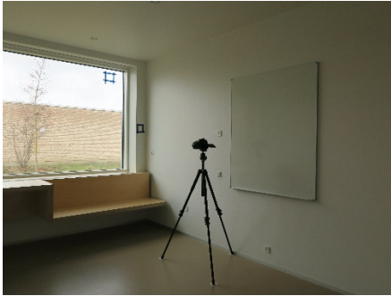
Figure 1-7 - Canon EOS 60D DSLR camera with a fisheye lens for luminance mapping
