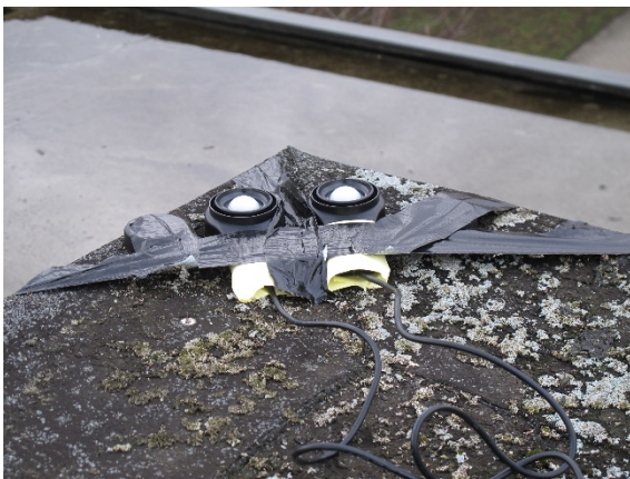
Figure 2-11 – Placement of the exterior illuminance data loggers on the roof
