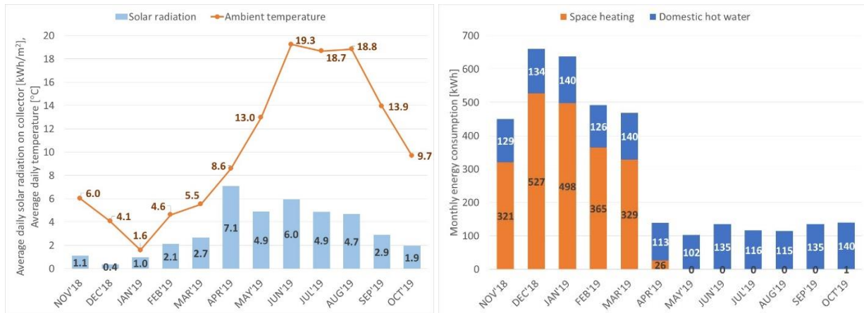
Figure 5. Measured weather data and energy drawn from HYSS in test period. Left: Solar radiation on solar collector and average ambient temperature. Right: Space heating and domestic hot water consumption.
