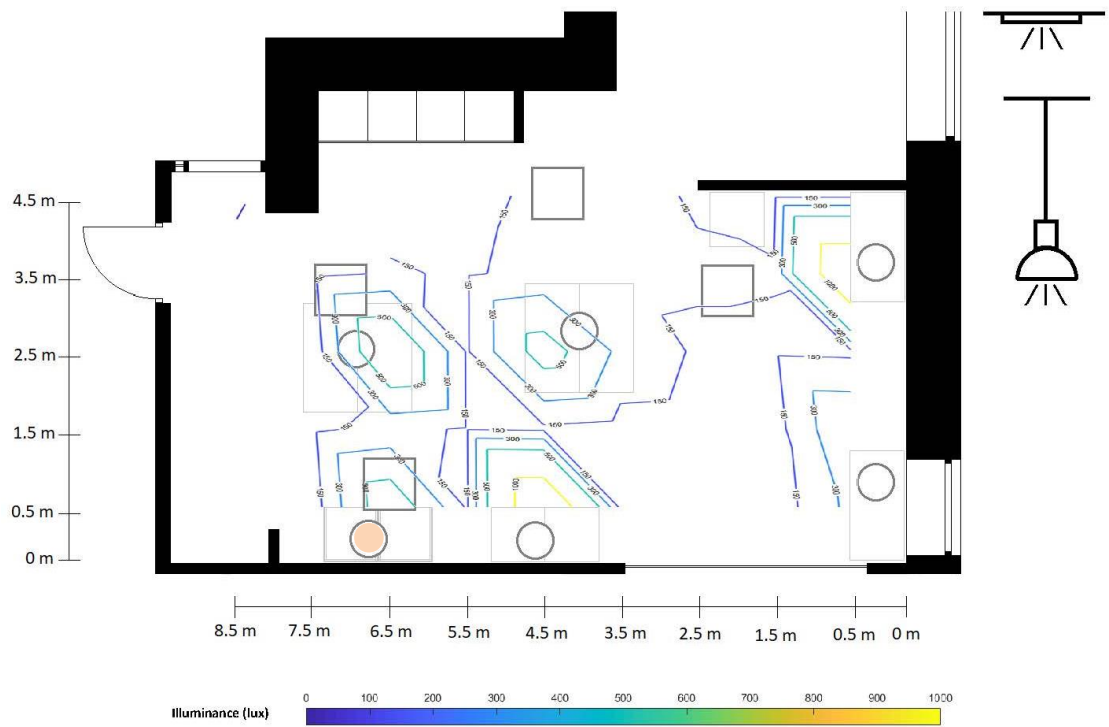
Figure 6.9: Illuminance levels [lux] at 0.6m above floor level in room 1.2.06 under New Scenario B – Ambient CL (30% output lighting) + Focused Pendants (100% output) for electric lighting only.
