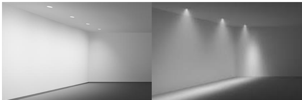
Figure 3.1: Type A uniform spatial light distribution
