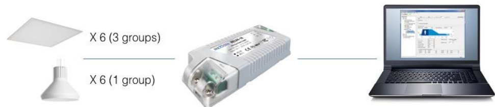
Figure 3.12: Energy monitoring setup
