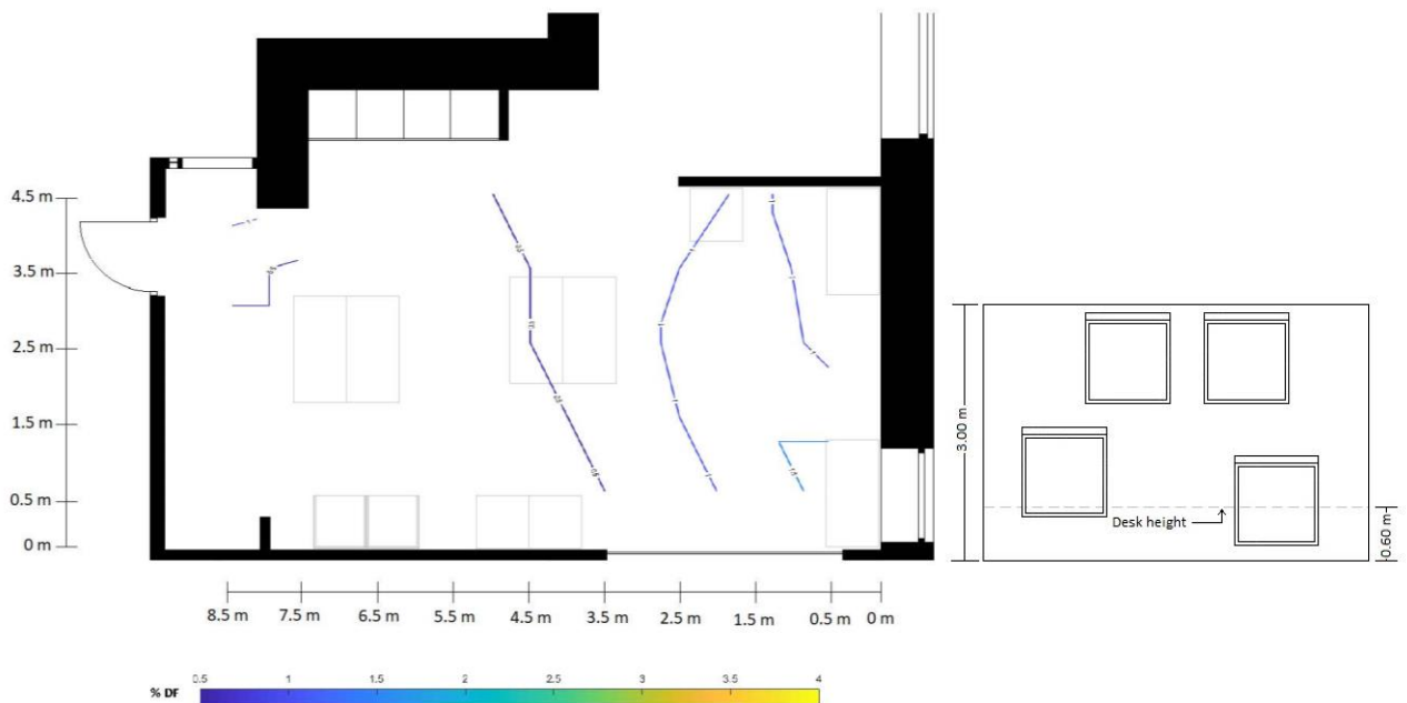
Figure 6.13: Daylight factor level [%] at 0.6m above floor level in room 1.1.10 (left). Façade window layout of the classroom as seen from outside the room (right). Glazing-to-floor-area-ratio = 18%
