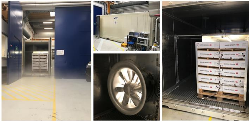
Figure 5: Selected images of the test setup at Danish Technological Institute. To the left a view into the open container. Middle upper is a side view of the container and the measuring equipment. Middle lower is the fan, and the one to the right is a view into the container looking at the third measuring pallet.
