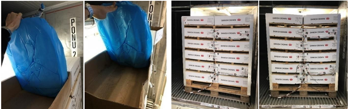
Figure 30: Illustration of the test change. To the left, a change in box structure. To the right, a change in air spacers.
