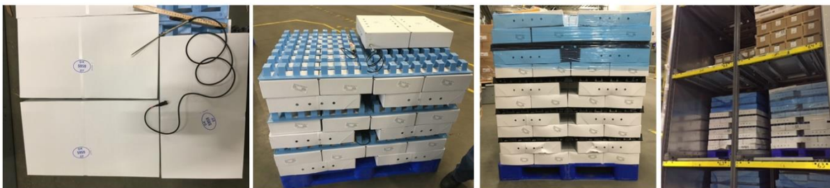
Figure 39: Illustration of the test setup at Claus Sørensen. From the left: Placement of the temperature sensors, pallet assembly, finished pallet, and placement in the tunnel.
